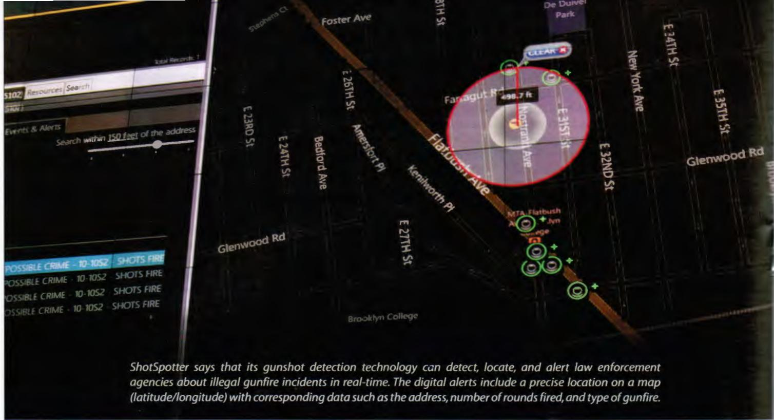
ShotSpotter says that its gunshot detection technology can detect, locate, and alert law enforcement agencies about illegal gunfire incidents in real-time. The digital alerts include a precise location on a map (latitude/longitude) with corresponding data such as the address, number of rounds fired, and type of gunfire.
